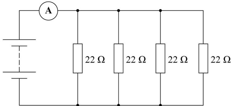
Show, using **Figure 12**, that the current in the power supply is about 0.25 A.
