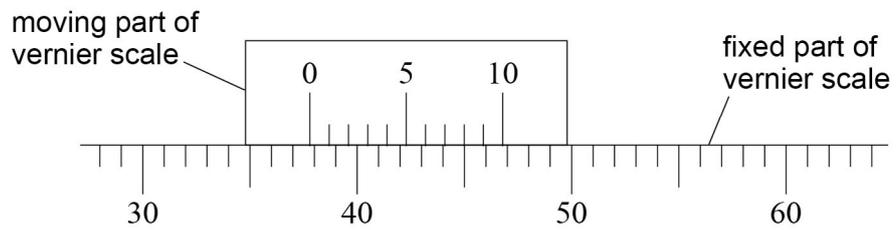
The smallest division on the fixed part of the scale is 1 mm.
