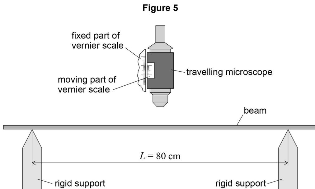
The beam is placed horizontally on rigid supports.
