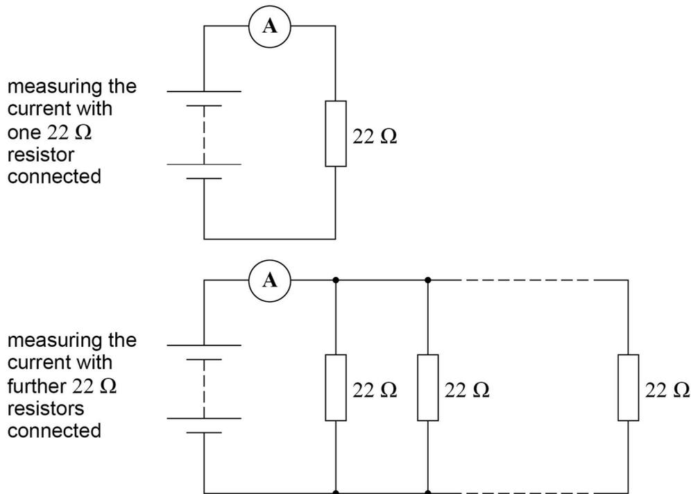
Initially the power supply is connected in series with an ammeter and a  $22\ \Omega$  resistor. The current  $I$  in the circuit is measured.
