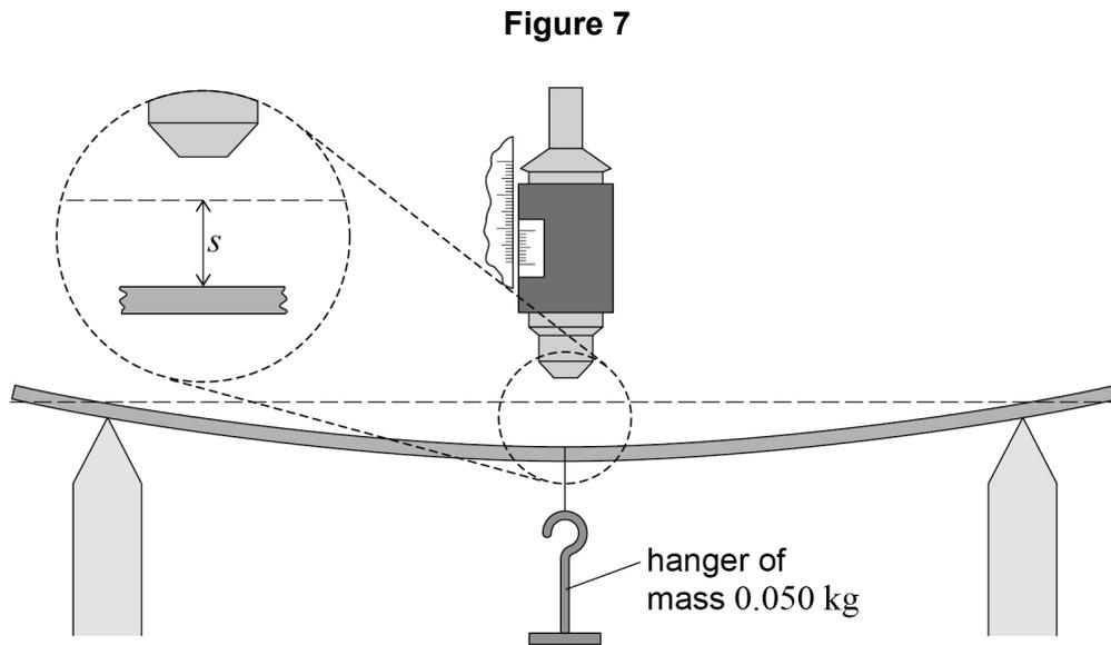
The microscope is refocused on the upper surface and the new vernier reading  $R$  is recorded.
